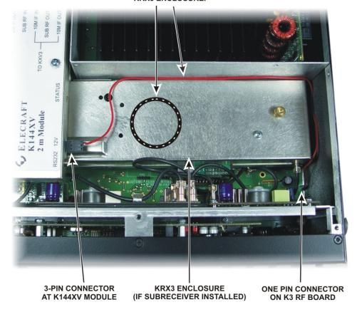
Figure 9. Installing K144XV Power Cable.
