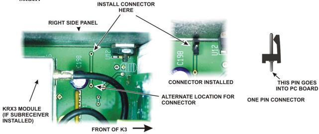
Figure 4. Installing the One-Pin Power Connector on the K3 RF Board.
