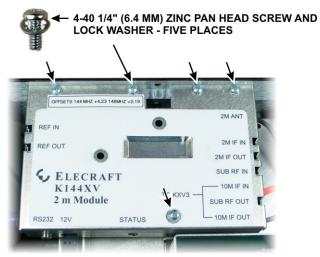
Figure 8. Installing the K144XV Module Top Cover.
