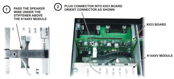
Figure 11. Connecting the Speaker Cable.
