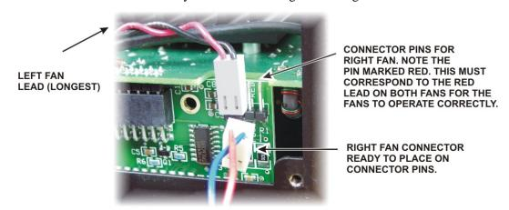
Figure 5. Reconnecting Rear Panel Fans on K3/100.
