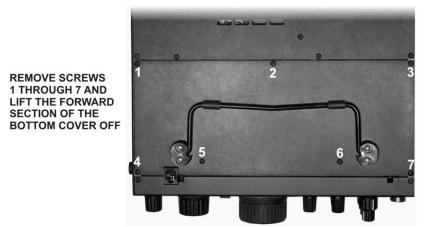
Figure 3. Removing K3 Bottom Cover.
