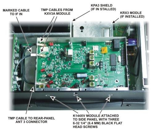
Figure 7. Mounting the K144XV Module in the K3.
