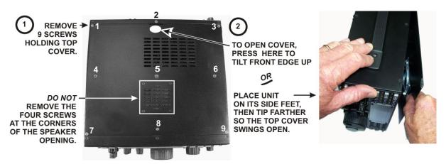
Figure 1. Removing K3 Top Cover.
